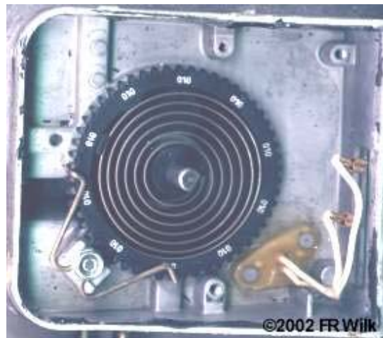
1. Wiper track 2. Wiper 3. Spring 4. Ring gear 5. Ring gear retainer 6. Temperature sensor 7. Wiper assembly retainer 8. Electrical connector 9. Bridge to wiper
