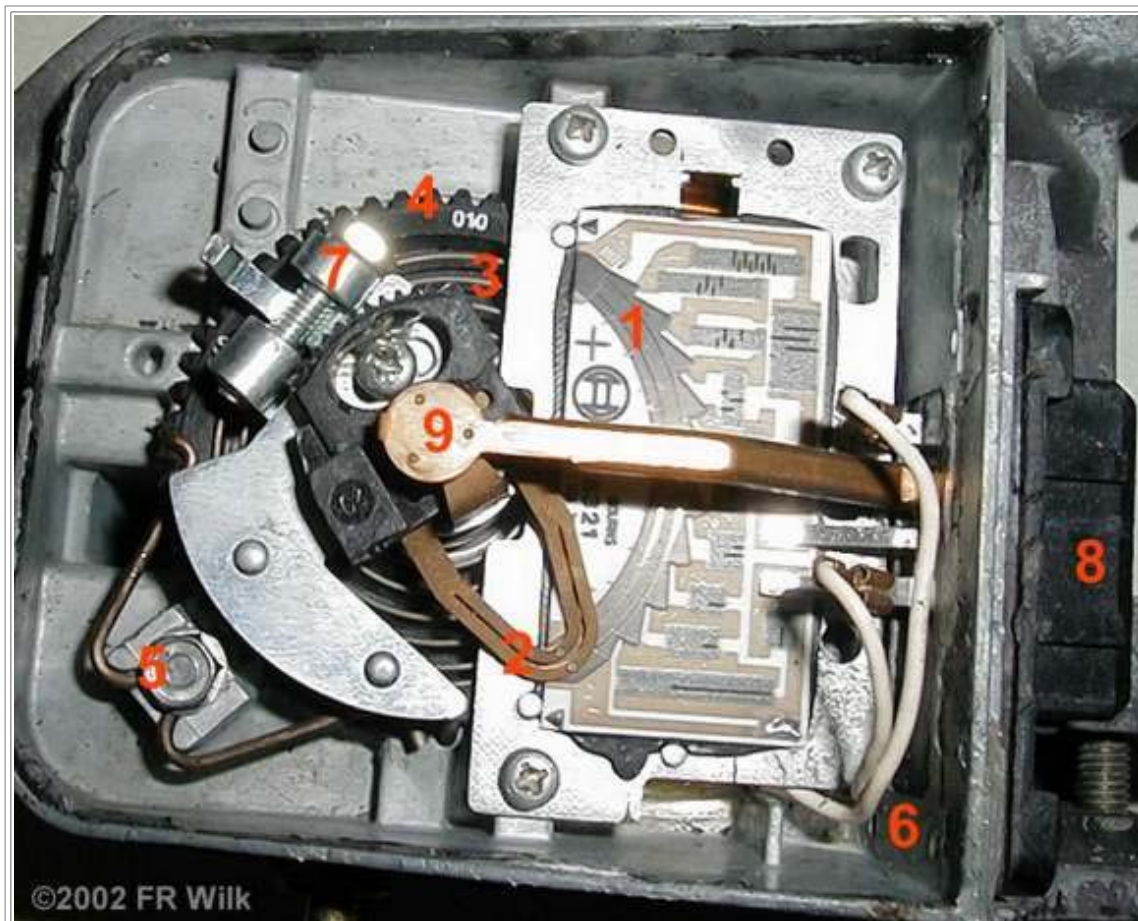
1. Wiper track 2. Wiper 3. Spring 4. Ring gear 5. Ring gear retainer 6. Temperature sensor 7. Wiper assembly retainer 8. Electrical connector 9. Bridge to wiper
