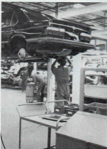
Final adjustments are made to a newly-installed rear suspension.
