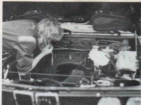
S-Series body shells arrive from the Dingolfing assembly plant less engines, transmissions, drivetrains, trim, and interiors. Here an "M Assembler" prepares a US M5 to receive its heart — the 3.5-liter 24-valve M Power.
