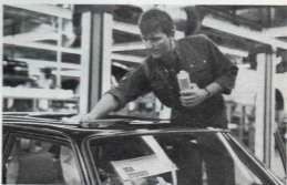
Completed cars are given a polish before being coated with Cosmoline for the trip across the Atlantic.
