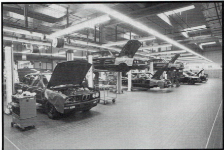
Final assembly of M5s is accomplished in a special BMW Motorsport shop north of Munich. A team of two technicians completes each car. It takes about three days to build an M5. Up to 20 cars are finished each day.
